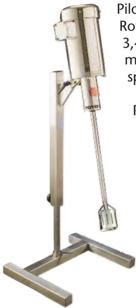
Pilot plant units (Rotosolver disperser model RS-02 and Rotostat emulsifier model XP-02) operate at up to 3,450 RPM with larger mix heads than our BenchMix models (refer to table below), providing the ideal tip speed and shear rate for many applications.
